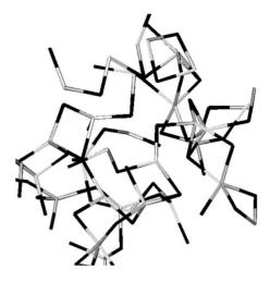
FIG. 1. Snapshot of the 120 atom liquid SnSe<sub>2</sub> at 1173 K. Selenium atoms are in black. Note the presence of edge-sharing units (four rings) in the structure.
