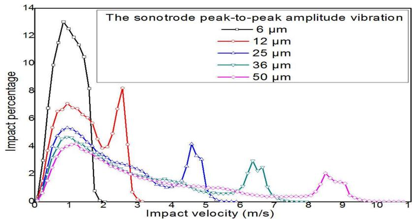
Fig. 7 - Influence of the sonotrode amplitude vibration on the impact percentage vs. impact velocity
