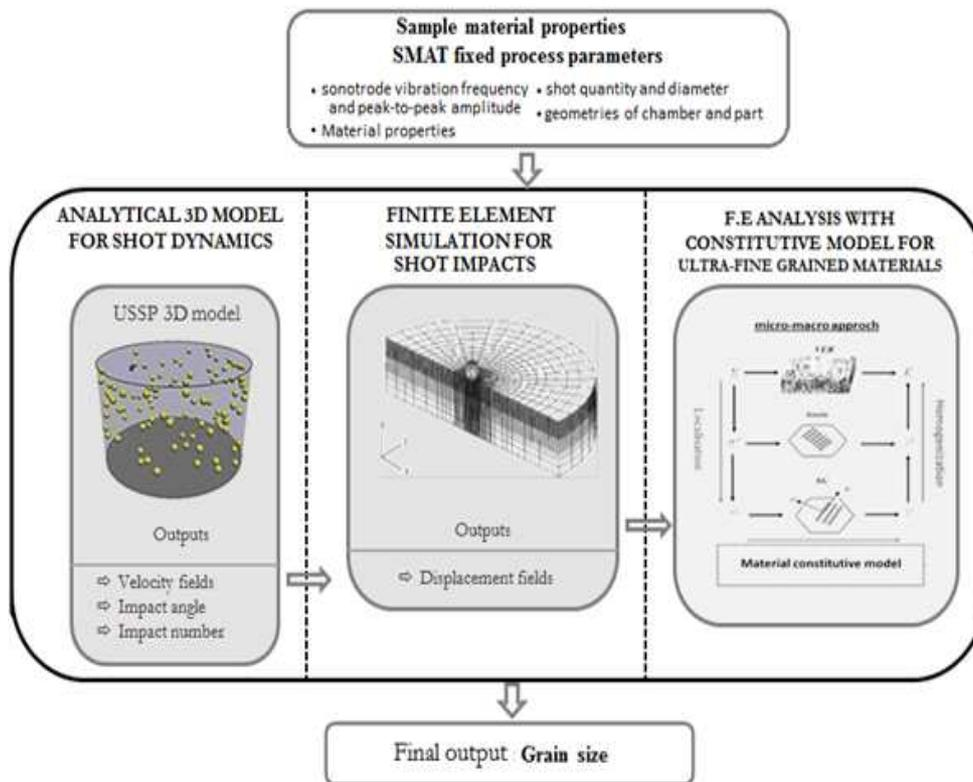
Fig. 1 - General numerical chaining methodology
