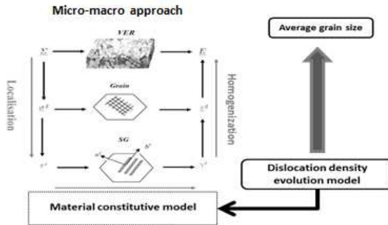
Fig. 9 - Micromechanical approach using a dislocation evolution model
