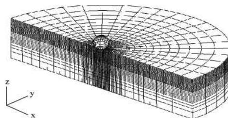
Fig. 8 - Three-dimensional FE model for a single shot impacting on a target.
