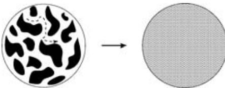
Fig. 7. Homogenisation of a diffusion process in a porous medium: particles, of diffusion coefficient D inside the pores, experience a hampered diffusive motion at larger scales; if the typical size of the pores is finite, normal diffusion is still observed, with lower diffusion coefficient D_{eff} , where D_{eff}/D is related to the medium porosity (Nicholson 2001; Laguës and Lesne 2003).
