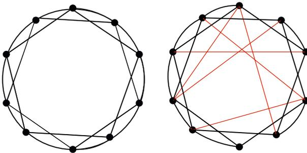
Figure 4. Watts and Strogatz model. Edges of a regular network are rewired at random (independently) with a given probability  $p$ , yielding a ‘small world’ of diameter increasing logarithmically instead of linearly with the number of nodes.
