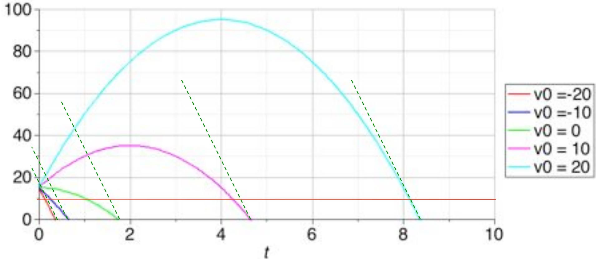
$$v_{z=0}^2 = v_0^2 + 2 g h$$
